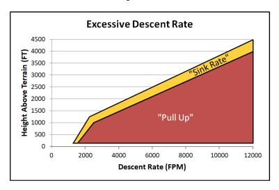
The "Pull Up" warning will provide up to 24 seconds of protection, while the "Sink Rate" caution will provide up to 33 seconds of protection, based on aircraft altitude. Aircraft vertical speed and current terrain elevation below the aircraft are used to compute the alerting altitude thresholds. As a result, these protection times may not apply in rising terrain or when the aircraft's rate of descent is increasing.
